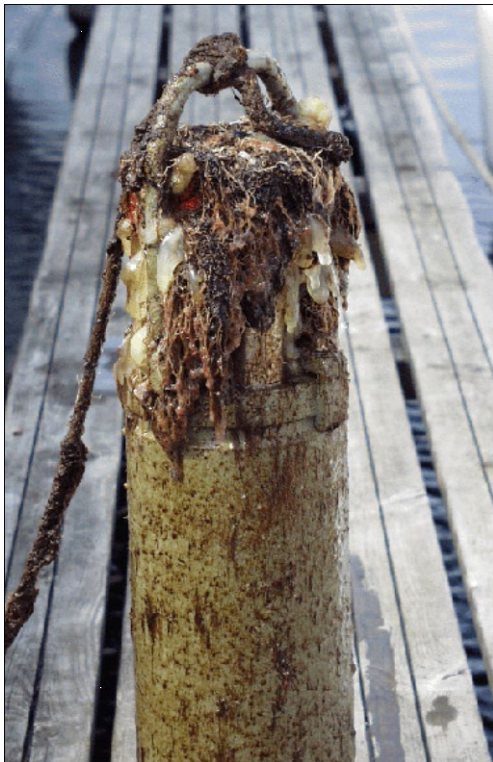
Figure 6-1: Example of fouling on an RCM 9 with an Oxygen Optode 3830 (Optode version with SR-10 output) mounted to it: The Optode was still giving correct readings.
