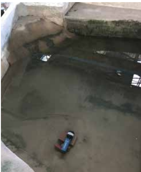
Fig. 1: SeaGuardII instrument tested in one of the hydraulic dam models
