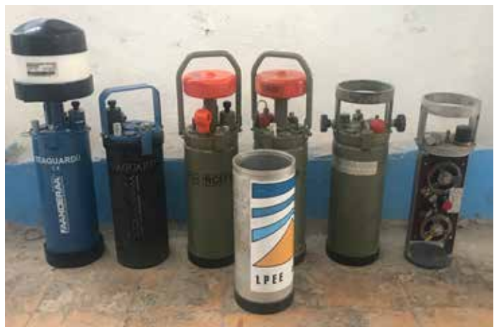
Fig. 2: Six generations of Aanderaa instruments at LPEE. From left to right: New SeaGuardII acoustic profiler/CTD/Wave instrument, SeaGuard Wave and Tide recorder (2007), Recording Current Meter 9 MkII (2000), Recording Current Meter 9 MkI (1996), Water Level Recorder 7 (1987), and Bottom pressure recorder with magnetic tape from the early 1980s. All instruments, but the last one are still in service.
