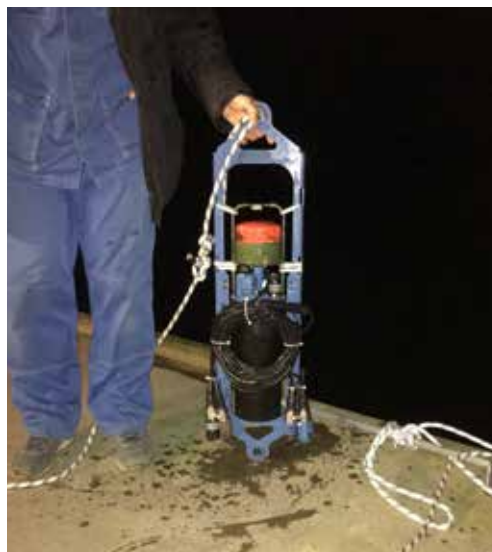
SeaGuardII prepared for gradient measurements with four sensors at bottom of frame and five sensors at top plate of the instruments.
