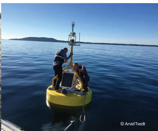
YSI EMM 2.0 buoy at test site outside Bergen
