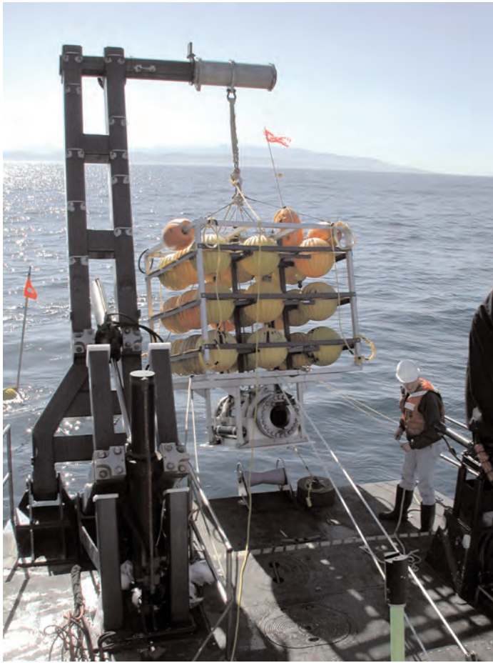
Fig. 4. The hyperbaric fish trap-respirometer during deployment in Monterey Bay from the RV Zephyr . The float rack contains 27 Benthos spheres and 3 cubic feet of syntactic foam.
