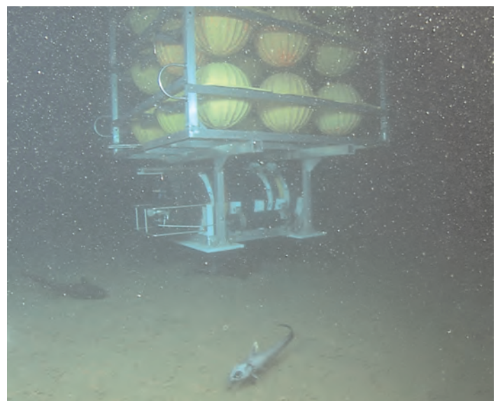
Fig. 6. The hyperbaric trap-respirometer on the seafloor at 1500 m. Two C. acrolepis can be seen, one is to the left of the trap and another is in the foreground.
