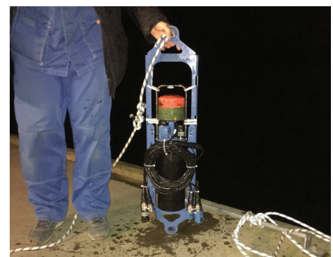
Figure [2]: SeaGuardII prepared for gradient measurements with 2*O 2 , 2*pCO 2 , 2*salinity/temp, 2*wave/tide and current.
