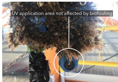
[3] Heavy biofouling is experienced after 3 months of deployment. However, Aanderaa Conductivity Sensor 4319 remains clear from biofouling as a result of Barnakil UV application on it.
