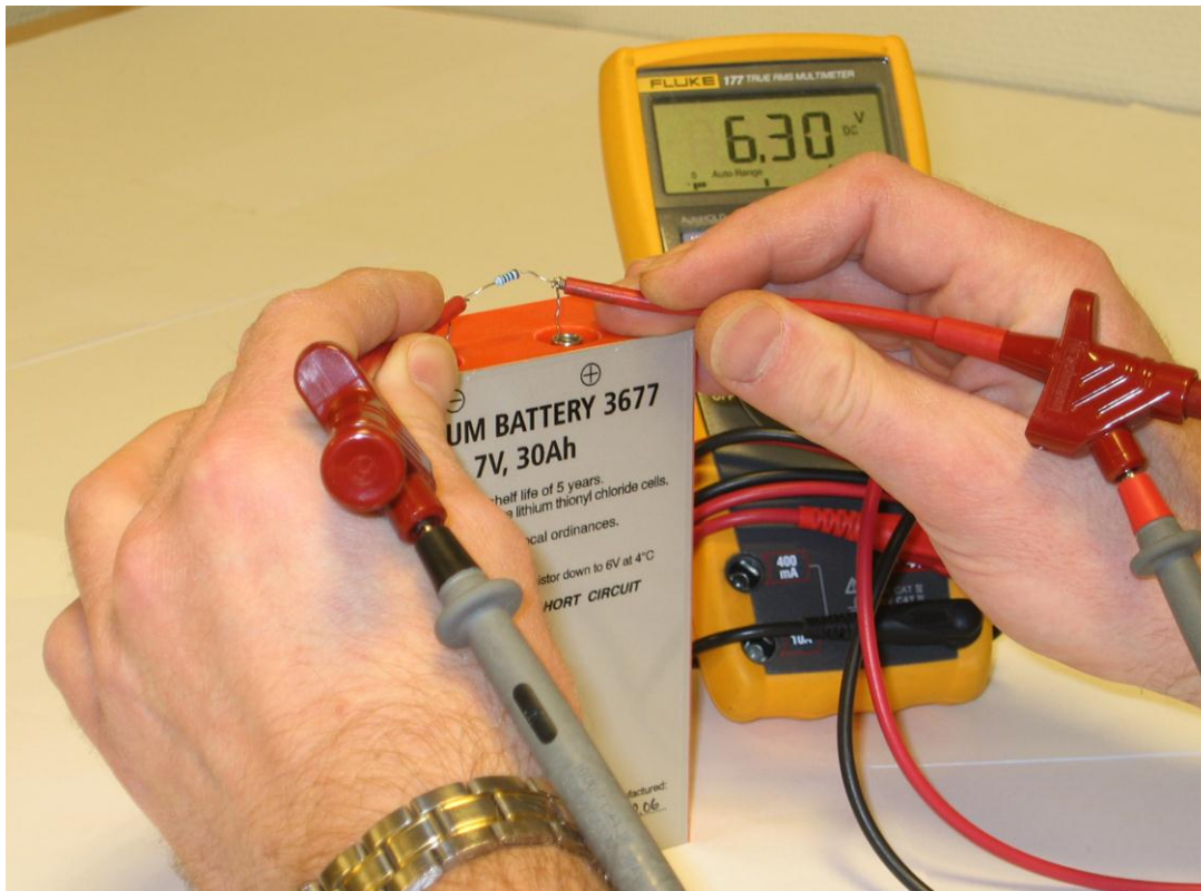
Figure 7-19 Use a 100 \Omega resistor up to 6.3 V to rejuvenate the battery.
