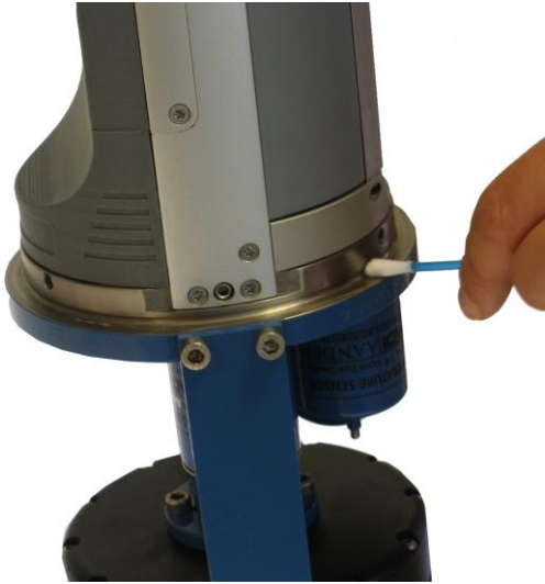
Figure 8-2 Clean O-ring seating; instrument up-side-down.
