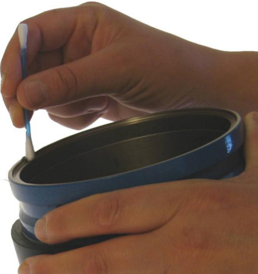
Figure 8-1 Clean O-ring seating.
