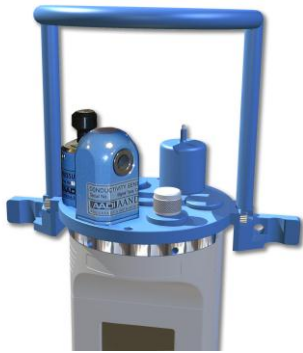
Figure 1-2 An example of the SeaGuard Platform configured as a CTD instrument.
