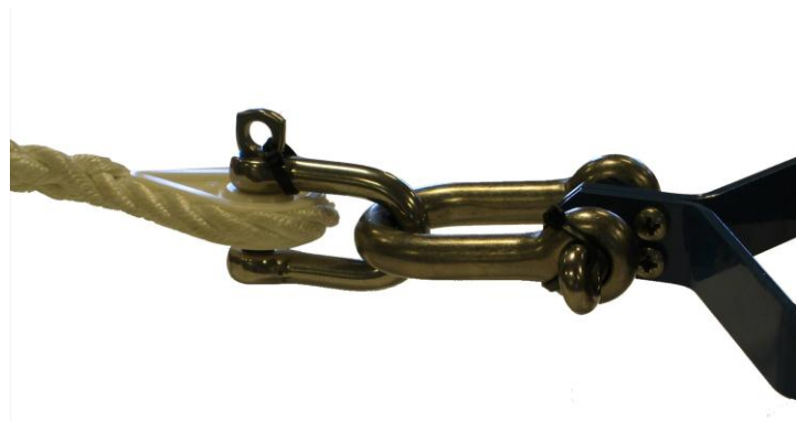
Figure 7-4 Splice the rope and fasten it to the thimble attached to the shackle.
