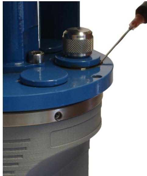
Figure 8-5 Add Tectyl® around sensors and sealing plugs.
