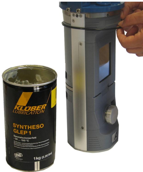
Figure 8-4 Lubricate O-rings with grease. (Klüber Lubrication Syntheso Glep 1 or similar synthetic grease).
