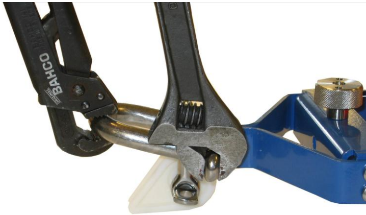
Figure 7-3 Fasten shackle in frame. Tighten thoroughly.
