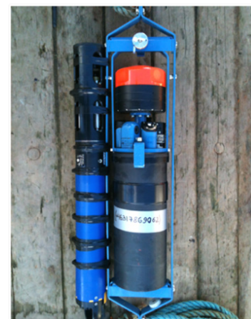
Figure 2: SeaGuard and EXO2 clamped together for the deployment
