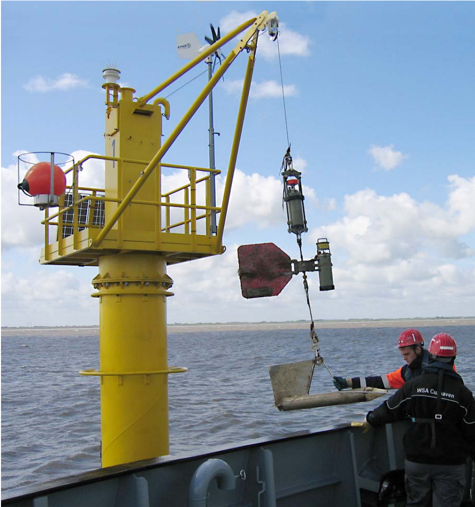
Deploying instruments on a River Pile Station.
