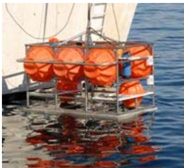
Fig.3 Illustrating the mooring rig system being deployed
